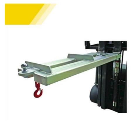
This slip on tow jib attachment with 2 hook positions and a tow ball fitted at the front of the jib. Both hook positions have a WLL of 2000kg. Not exceed 500kg when use the tow ball and the minimum capacity of the forklift is to be 2 tonne. Locking pins provided to prevent the jib from moving off the fork arm. Galvanized finish.
