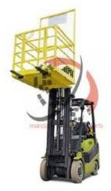
\*\*\*Please note the use of this work platform on a forklift truck should not be considered if the capacity of that forklift is less than 1860kg for a counterbalanced type or 1116kg for a reach type Forklift.\*\*\*
